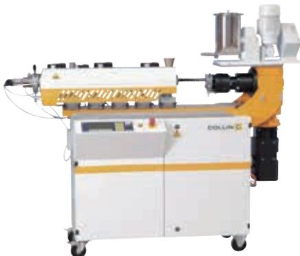
The Collin Compounder Type E Entrance is perfectly suitable for easy compounding tasks. The free-standing machine can connect different polymers in various ways and is very flexible when it comes to dosing – side feeders, volumetric or gravimetric dosing units. The compounder also shows flexibility with the downstream equipment, which can range from a water bath or pelletizer to a small blown film line or cast film line.
