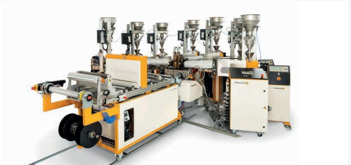
The base unit consists of two horizontally arranged chill rolls, suitable for cast films within a thickness range from 20 to 300  $\mu\text{m}$ . Collin adapts the speed and roll-diameter of the chill rolls according to the customer's needs. Downstream equipment can also be implemented flexibly – depending on the requirements, different types of take-off rolls, edge cuttings, measuring instruments or unwinders and winders.
