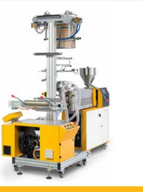
The version Blown Film Line E is the entrance version and is particularly used for quality control. This line has got a central column with a fixed overall height and a simple mono cooling ring.
