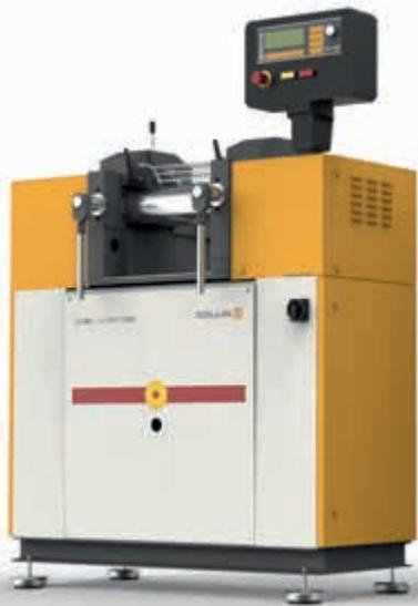
The roll mills are used for mixing, plasticising, kneading or laminating of plastics and are simple roll mills with manual gap adjustment. This is why the E for Entrance series exists as useful alternative for laboratory and pilot tests.
