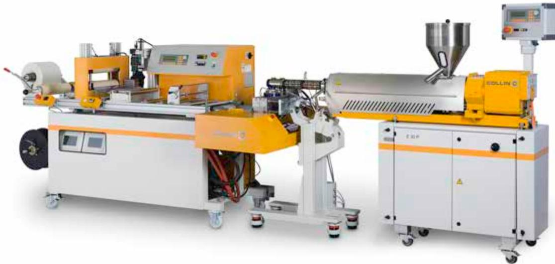
These versions combine finishing calender and the chill roll and are used for the production of thin-walled or double-wall films. The 3-roll unit can be used for vertical or horizontal operation. The forces in the polishing gap can be created in a hydraulic or pneumatic way. The polishing roll is suitable for a wide range of applications such as smoothing, embossing or laminating.
