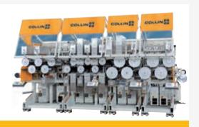
The stretching of polymer films improves their characteristics in a variety of ways. Collin stretching lines consist of an extrusion group, the stretching unit, take-off and winder.
