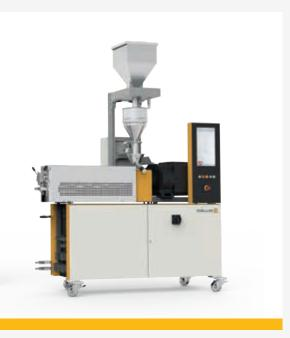
The high-speed machines of the Type T extruder series unite the advantages of Type P, however, due to the strongly increased speed at a high drive torque, the output is essentially higher. Especially the development of the screw geometry and the feeder for the high-speed machine required enormous technical competence.
